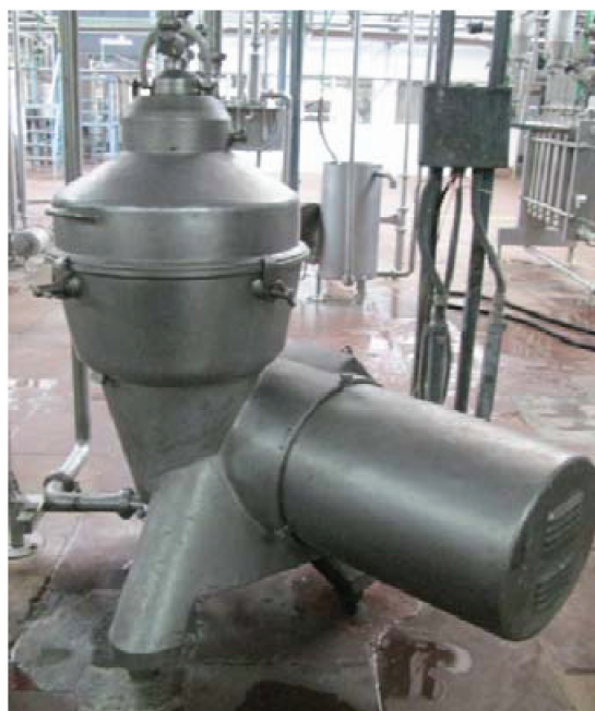
Fig.3.5. In-line modern clarifier
