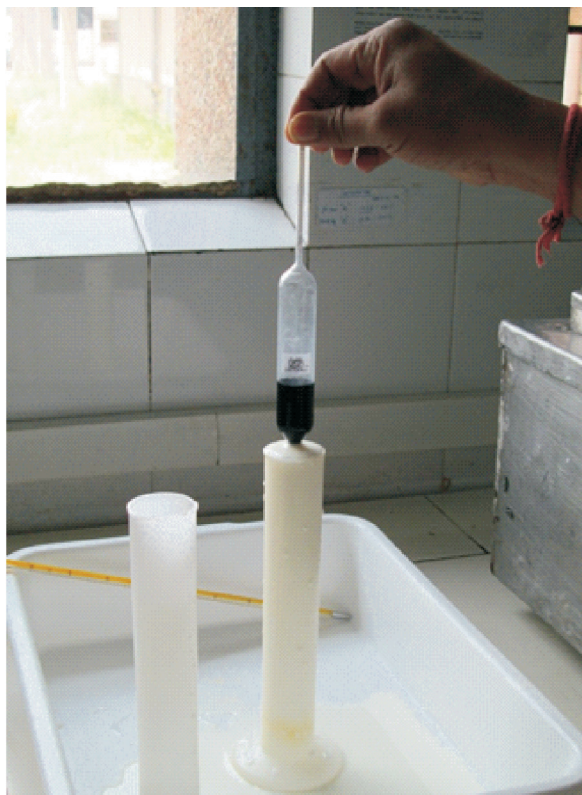
Fig.2.1. Measurement of density of milk using lactometer
