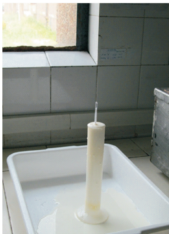
Fig.2.1. Measurement of density of milk using lactometer
