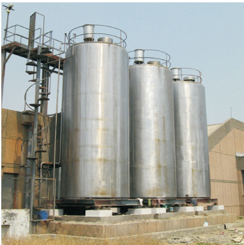
Fig.1.4. Milk storage silos
