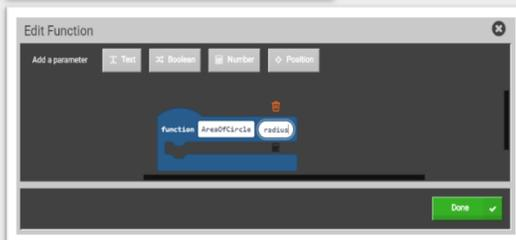
Step 6: Create a function with name “AreaOfCircle” having one numerical parameter named radius
