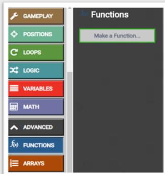
Step 5: Go to block type **FUNCTIONS** and click on “**Make a Function**”
