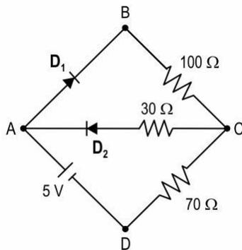
If the maximum current that can flow in either of the diodes is 30 mA beyond which they burn out, determine which of the diodes are safe in the above circuit?
