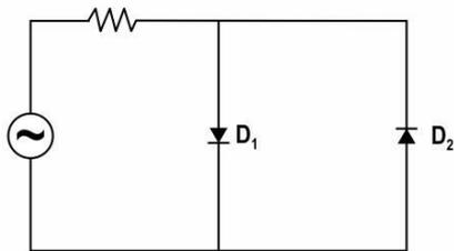
(b) Consider a network ABCD containing two identical diodes  $D_1$  and  $D_2$ . The two diodes offer a resistance of  $30 \Omega$  when in forward bias and infinite resistance when in reverse bias.
