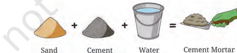
Figure 6.7: Mortar is made up of sand, water, cement and lime – it is more flexible than concrete, as it allows for slight movement without cracking.
