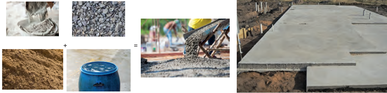
Figure 6.8: Concrete is made up of sand, water, cement, and gravel or crushed stones – it is a strong and durable building material that hardens over time, getting a stone-like quality.
