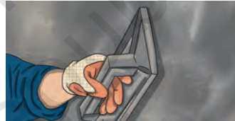
Float: It is used to flatten the plaster.
