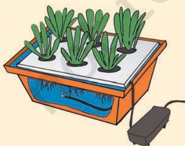
Figure 1.8: Growing plants using DWC hydroponic system
