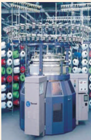
Figure 4.3- Circular knitting machine
