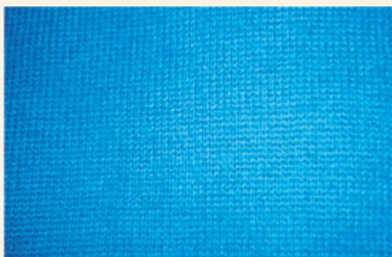
Figure 4.1- A weft-knitted fabric
