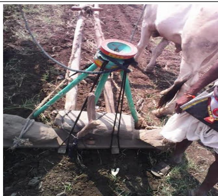
Figure 20 - Seed sowing plough with two seed bowls
