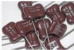
Some 1nF × 500VDC rated silver mica capacitors
