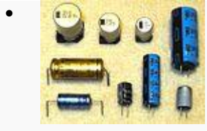
Axial, radial (single ended) and V-chip styles of aluminum electrolytic capacitors
