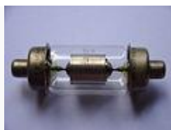
Vacuum capacitor with uranium glass encapsulation
