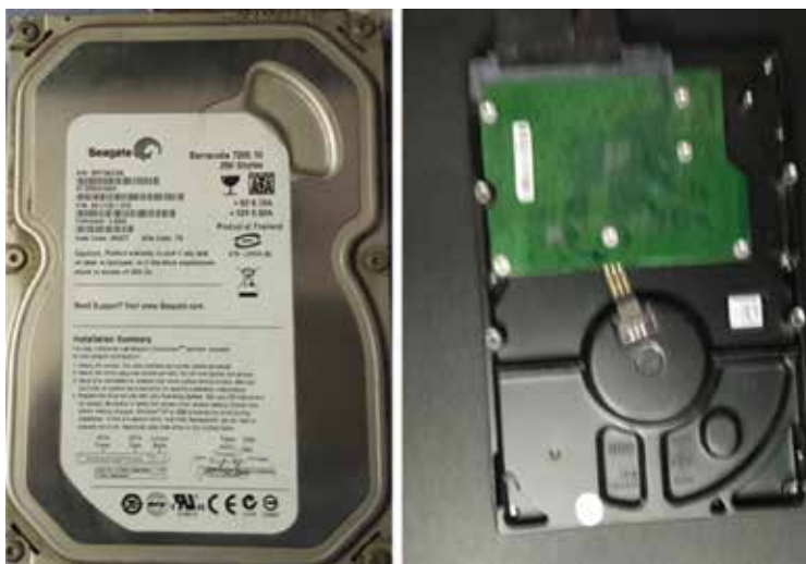
Figure 1.5: Two sided view of a sealed hard disk unit
