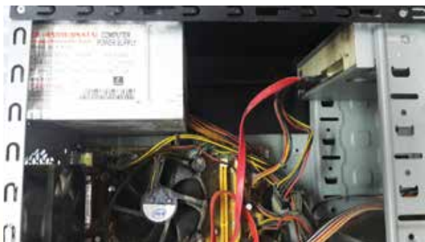
Figure 1.4: Power Supply Unit
