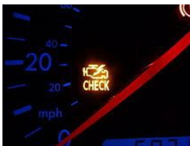
A MIL "Check Engine" light on a Volkswagen Bora indicating a fault in the Engine Management System.
