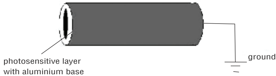
Fig. 13 Photosensitive Drum with aluminium base
