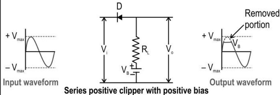
During the positive input half cycle, the diode is reverse biased by the input supply voltage  $V_i$ . But since the positive terminal of the battery is connected to p-side and the negative terminal of the battery is connected to n-side of the diode, the diode is forward biased by the battery voltage  $V_B$ .
