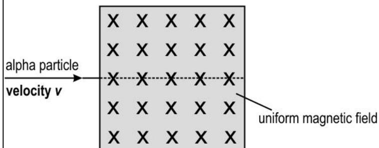
A uniform electric field is applied in the same region as the magnetic field so that the alpha particle passes undeviated through the combined fields.
