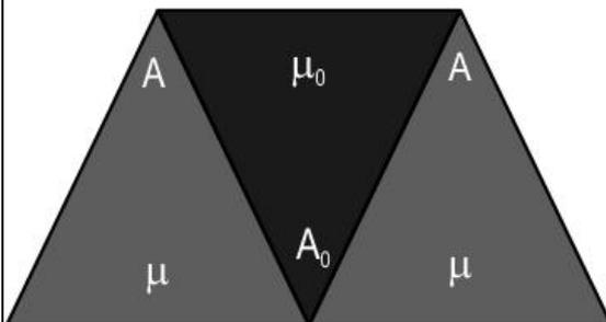
Prove that for a net deviation produced in the light ray to be zero,  $\mu = \mu_o$  in the given combination.
