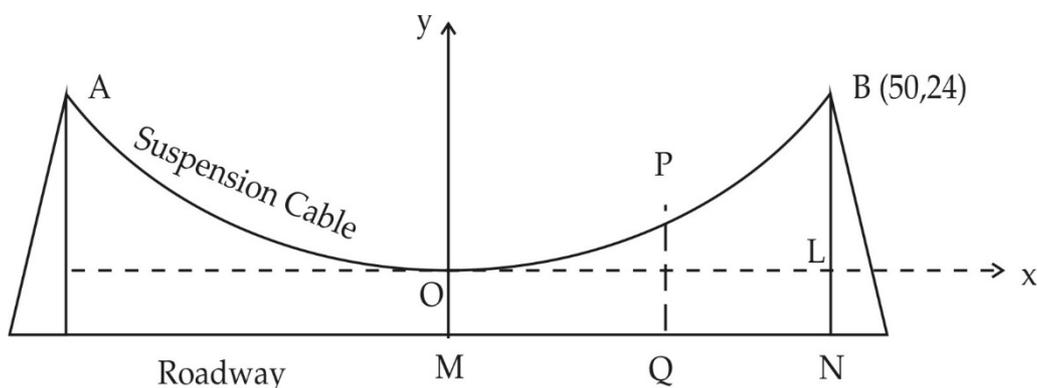
The bridge is hung by supporting wires in a parabolic arc with vertex at the lowest point and the axis vertical. The equation of the parabola can be taken as
