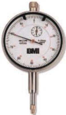
It works on the rack and pinion principal. The plunger has gear teeth cut on it and when it reciprocates it actuates a pinion attached to the pointer shaft. Thus any movement of the plunger causes a corresponding movement of the main pointer on a graduated dial.
