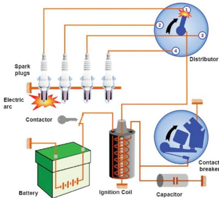
When the ignition switch is 'ON' the current flows from the battery through the primary winding and produces a magnetic field in the coil. When the contact points open the magnetic field 12 volts from the
